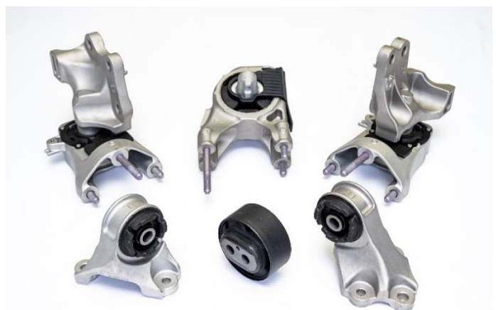
eAxle mounts: Front three for the rear and back three for the front.
