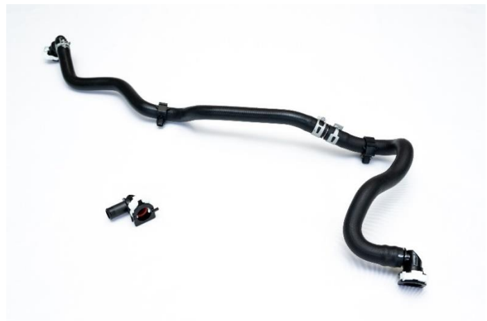
Cooling hoses and connectors for the electric system (front left)
