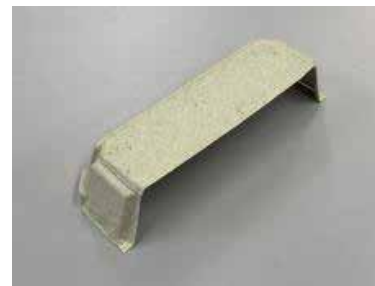
Prototype with a small mold ⇒ Good shape followability
