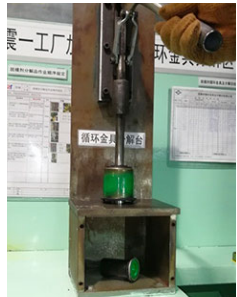
Workbench for dismantling vulcanized products
